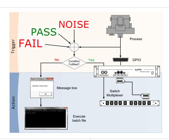
The IO & Prompt is a complementary task of the KLIPPEL QC software designed for the conditional interaction with an automated environment and the QC operator during a test sequence.
