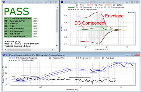
The upper right chart shows excursion-based results derived from the measured waveform of a typical micro-speaker. In this example the dynamic coil position (labeled: DC Component) is checked against constant, user defined limits.
