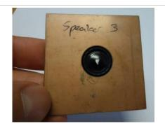
The outer dimension of the panel should be between 50mm and 70mm. A ring with inner diameter of 45mm is used to press the panel on a sealing ring.
