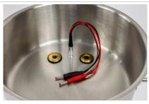
The inner cable is equipped with two 4 mm male laboratory connectors with removable shells. The FORCE and SENSE wires are connected inside the laboratory connectors, as close as possible to the DUT.
