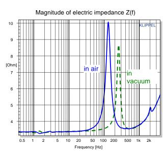
The lumped parameters of the mechanical system (moving mass  $M_{ms}$ , stiffness  $K_{ms}$  and mechanical resistance  $R_{ms}$ ) can be measured more accurately by performing the measurement in vacuum. Comparing the pure mechanical parameters with the parameters measured in air allows to separate the contribution of the air to the measurement in free air.
