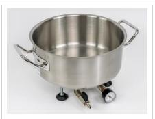
A cylindrical vessel made of low magnetic stainless steel can be loaded by most kind of transducers such as woofers, tweeters, horn compression drivers, headphones and micro-speakers. The low magnetic material used will not affect the magnetic properties of the transducer. Only transducers with very strong outer B-field should be isolated from the chamber by some millimeters of air distance.
