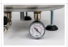
A pressure manometer shows the pressure difference between the interior of the vacuum chamber and the ambience in bar.
