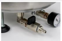
The air in the vacuum chamber is exhausted via a tap on the bottom of the vacuum chamber. The hose connected with the vacuum pump can be easily removed by using a fast coupler system.
