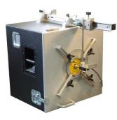
Fold down the laser rack and adjust the laser head
