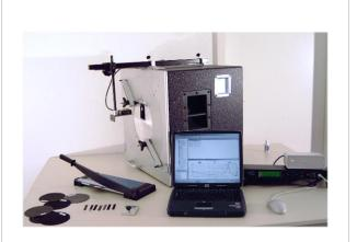
The material parameter measurement module (MPM) measures the Young's E modulus and the loss factor  $\eta$  of the raw material used for loudspeaker design. The vibration beam technique (ASTM E 756-93) is modified to be capable for measuring also soft materials such as thin foils of plastic, rubber and any kind of paper and impregnated fabric. After cutting 1 cm strips the probes are clamped on one side and excited pneumatically by using the suspension part measurement bench.
