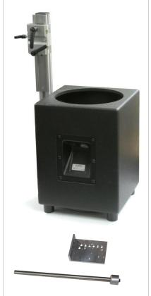
The LST Measurement Bench consists of a sealed enclosure with a volume of 26 liters and a 10" driver that excites the device under test (DUT) pneumatically.
