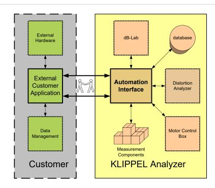
The Klippel Automation Interface provides a Software API to access individual components of the Klippel R&D System in a variety of client programming environments and scripting containers.
