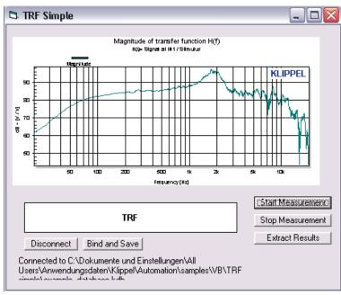
This example may be executed after installing the setup and starting *Operating\_TRF\_via\_VB6.exe* from the start menu under *Klippel Analyzer/Automation/samples*. The visual basic code (60 lines only) is described in the user manual of the automation interface.
