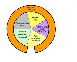
The Klippel Automation Interface provides programmers access to Klippel measurements and simulations and to the databases that store settings and results. The COM/ActiveX interface can be used in many programming and script environments, such as Visual Basic 6, Visual Basic.NET, C#, Delphi or other containers like Microsoft Excel.
