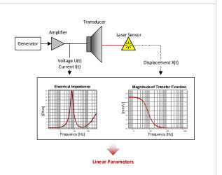
of the loudspeaker model at low frequencies. The LPM provides tools to identify and avoid typical problems such as poor signal to noise ratio and malfunction due to nonlinear effects of the driver or amplifier limiting.
