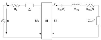
Figure 1: Equivalent electrical circuit for air measurements
