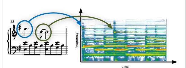
Based on three different methods, the Wavelet Transform (WT), the Short Time Fourier Transform (STFT), or a Bark scaled Filter Bank Transform (FBA), the module decomposes the input signal and visualizes the signal characteristics over frequency and time.
