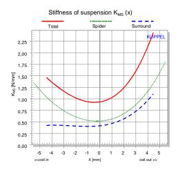
The graph compares all three stiffness curves, which allows a detailed investigation of the separated contributions towards the total stiffness. Note that the remaining surround material will partially influence the spider stiffness characteristic. However, in most cases, the surround is softer than the spider resulting in a minor influence. Further information on how to improve the suspension linearity may be obtained from the Application Note AN3: Adjusting the Mechanical Suspension.
