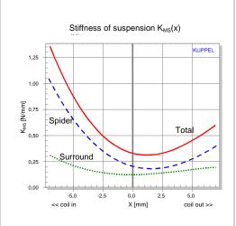
In this example, since the surround characteristic is very flat and much softer than the spider, the asymmetry in the spider clearly dominates the total stiffness. The surround has almost no influence on the asymmetry of the total stiffness. In the suspension's current rest position, shown at x=0 in the graph, the spider material is stretched and it droops slightly inwards (towards the magnet.)
