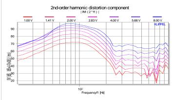
At low and medium voltages the 2<sup>nd</sup> order distortion component raises by 6 dB revealing a quadratic relationship. The increase stagnates at the last voltage step.
