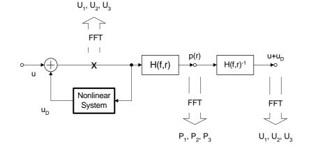
By performing a filtering of the input measured sound pressure signal with the inverse system function  $H(f)^{-1}$ , the effect of the radiation and room interactions can be compensated and the equivalent harmonic distortion
