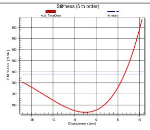
The stiffness curve K(x) versus displacement is shown in the figure. For a positive displacement x=+11 mm the stiffness is approximately 30 times higher than at the rest position x=0. Please note the distinct asymmetry of the curve. The stiffness at negative displacement x=-11 mm is only 16 % of the stiffness at positive displacement x=+11 mm. Under dynamic operation an ac-signal is partially rectified and a negative dccomponent is generated. The dashed blue curve shows the
