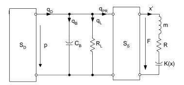
The driver generates a volume velocity  $q_D$  that divides into three parts as shown in the equivalent circuit above. The volume velocity  $q_B$  flows into the volume of the box,  $q_L$  is leaving the box through leaks and the volume velocity  $q_{PR}$  produces the force F driving the suspension part under test
