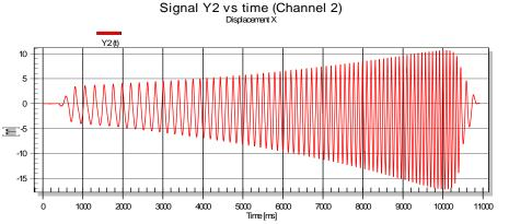
The window **X(t) Displacement** shows the displacement time signal swept from 4 to 12 Hz. The displacement rises slowly up to [-16...+10] mm peak but decreases rapidly after the resonance. This is caused by the suspension nonlinearity which causes a bifurcation and a jumping effect to lower amplitudes. The time signal also reveals a dc part in the displacement generated by the stiffness asymmetries of the suspension.
