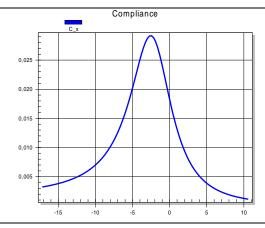
Activating the window **C(x) Compliance** shows the nonlinear compliance C(x) versus displacement x which is identical with the inverted stiffness. Note that the stiffness curve reveals the limiting effect more clear than the compliance curve and is more recommended for graphical representation.
