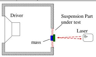
The figure above shows essential parts of the measurement setup. An 18" driver is mounted in a sealed enclosure having a second hole where the suspension part under test is placed. The outer rim of the suspension part is firmly clamped by rings.
