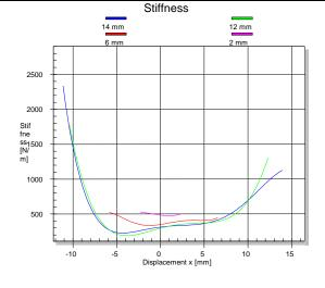
The dynamic measurement technique also reveals the dc displacement caused by asymmetries of the suspension. The ac displacement is partly rectified and produces a dc component which operates the suspension at a region of lower stiffness. The example shows a positive dc-displacement of 1.5 mm generated by a cone where the surround has a significant asymmetry at negative displacement.
