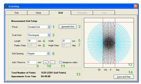
It is possible to enter the **Length (4)** and **Width (5)** of the driver and the grid points outside of that rectangle will not be measured.
