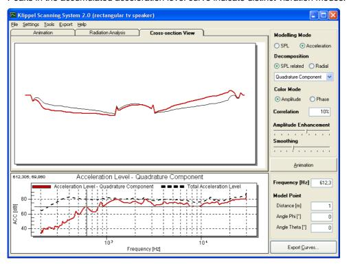
Peaks in the quadrature component curve of the acceleration level indicate vibration modes which do not contribute to the sound pressure output at the selected observing point in the far field, especially rocking motion at lower frequencies.
