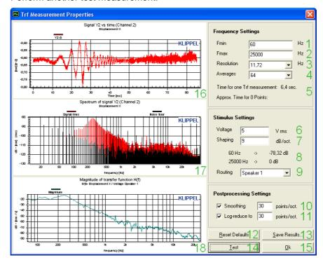
You can see that the signal to noise ratio (SNR) in the **Displacement Spectrum** (17) has decreased. That is due to the applied stimulus shaping. The given **Voltage** (5) input is applied at the highest frequency **Fmax** (5) and reduced towards lower frequency **Fmin** (1) according to the specified **Shaping** (7). Because Fmax has increased now from 10kHz to 25kHz the actually applied voltage at low frequencies has decreased.
