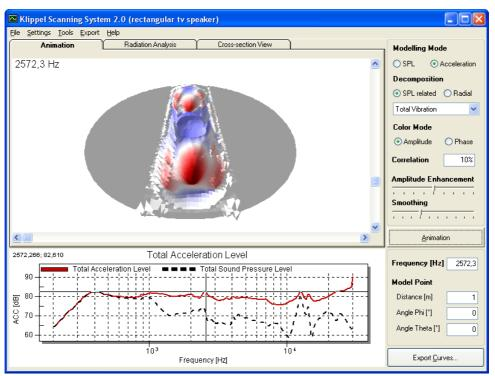
The vibration behavior can be studied over the complete measured frequency range. Peaks in the accumulated acceleration level curve indicate distinct vibration modes.
