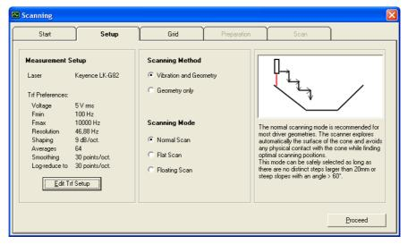
A first test measurement of the driver is advisable to find a good TRF measurement setup.
