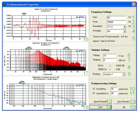
The setting of the stimulus voltage is important to get a good SNR. You can safely increase the voltage and reduce the shaping as long as the actual displacement as shown in the **Displacement Chart (16)** is small enough.
