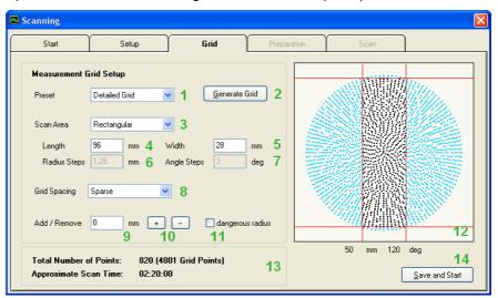
Now it is possible to increase the grid density again by switching to **Manual Grid Preset (1)** and reduce the **Radial Steps (6)** and **Angle Steps (7)** until the desired number of measurement points and scan time is reached.
