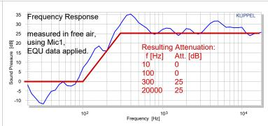
See the QC user manual in section Optimizing Performance / SPL Tests / How to cope with ambient noise? / How to measure Box attenuation? on how to calculate the specific ambient noise attenuation of the test box and how to set up the test setup considering this attenuation.
