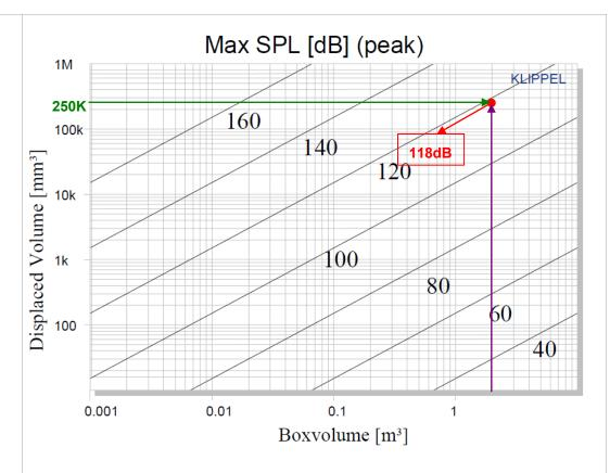
The figures above show an example for testing a subwoofer with a diameter of 140 mm and 18 mm peak displacement. The resulting peak SPL is about 118 dB. An optimal microphone for this application is the MIC255 (AN 2400-009) ½" type.
