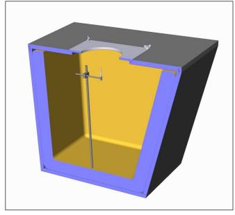
All walls should be equipped with sound attenuating foam of about 10 cm thickness to attenuate high frequency noise.
