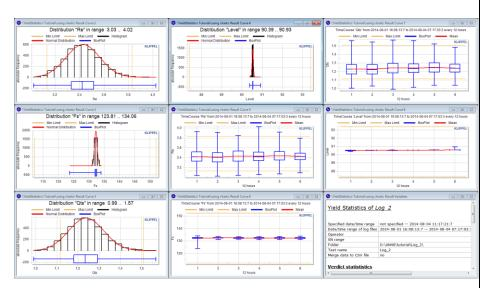
Note: outliers and invalid measurements may result in strange plots due to high result ranges. An example: The distribution plot of Re may be destroyed by not connected or shortened measurements (resulting in very high or low Re values). Please refer to the documentation on how to apply filters for the plots.
