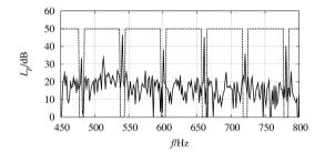
Fig. 4: Attenuation of the deterministic distortion components of a sound pressure spectrum (solid line) by a linear comb-filter  $H_{\text{stoch}}(j\omega)$  (dotted line, scaled).
