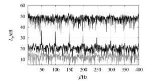
Fig. 9: Demodulated sound pressure spectra  $F\{p_{stoch}^2(t)\}$  simultaneously measured in the near (black curves) and far field (gray curves) of the test object; lower curves: silent environment, upper curves: ambient noise corruption
