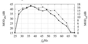
Fig. 15: Absolute (solid line) and Relative (dotted line) Modulation Level vs. excitation frequency for a vented box with leak
