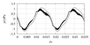
Fig. 1: Multiple waveforms of the sound pressure signal measured at a leaky enclosure (solid lines) and a sealed enclosure (dashed line) using a sinusoidal stimulus at 60 Hz (lower picture), far below the system resonance.
