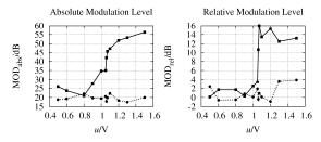
Fig. 11: Absolute and relative modulation level vs. excitation voltage, measured with (solid line) and without leak (dashed line) on a sealed box system
