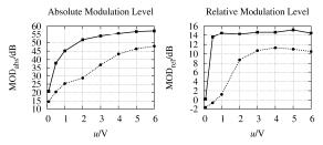
Fig. 16: Comparison of Absolute (left) and Relative (right) Modulation Level of isolated leak noise (solid line) and port turbulences (dashed line) measured at vented box system
