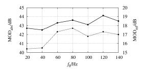
Fig. 13: Absolute (solid line) and relative (dotted line) modulation level vs. excitation frequency for a closed box system
