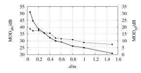
Fig. 14: Absolute (solid line) and Relative (dotted line) Modulation Level vs. measurement distance for a closed box system
