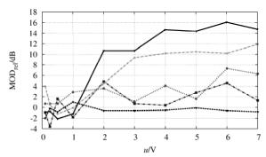
Fig. 17: Relative Modulation Level vs. excitation voltage at four different microphone positions around a large subwoofer with one leak and a reference curve without leak (lowest dashed line)
