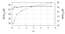
Fig. 12: Absolute (solid line) and Relative (dotted line) Modulation Level vs. measurement time for a closed box system
