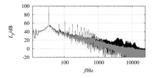
Fig. 2: Amplitude spectrum of sound pressure signal measured in the near field of a leaky (black curve) and sealed (grey curve) loudspeaker enclosure.
