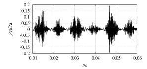
Fig. 5: Waveform of the stochastic distortion signal  $p'_{\text{stoch}}(t)$  extracted by comb-filtering The squared envelope signal
