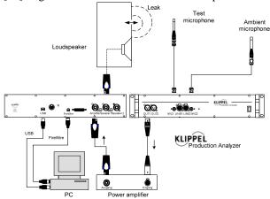
Fig. 10: Measurement setup with KLIPPEL QC System
