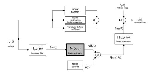
Fig. 3: Signal flow chart describing the generation of turbulent air leakage distortion
