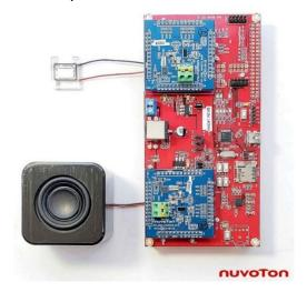
Both NAU83G10 and NAU83G20 devices have on-chip and low latency Tensilica HiFi Audio DSP, a high quality 24bit audio ADCs for current and voltage sense, and a battery tracking and brownout prevention ALC which are optimized for Klippel Controlled Sound (KCS) technology.
