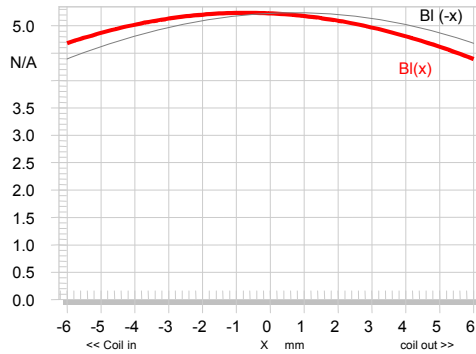
Figure 41: Force factor Bl(x) versus displacement of speaker 2 (thin curve shows mirrored Bl(-x) -characteristic)
